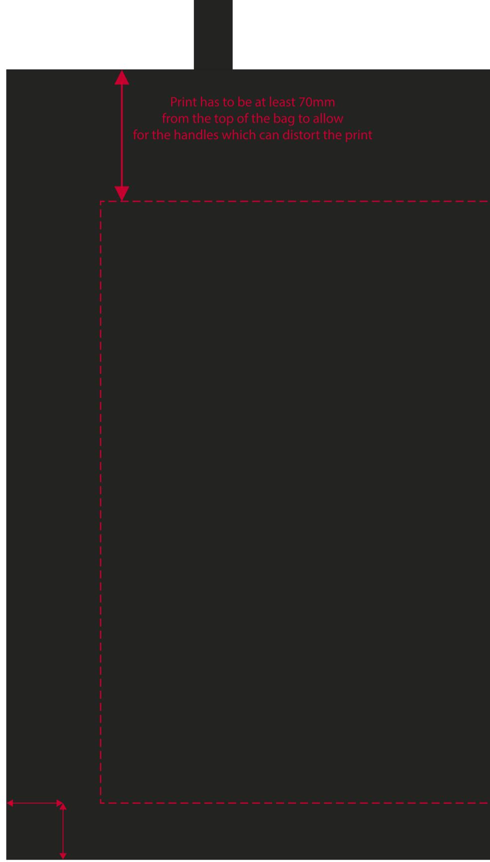
The closest we can print to the edge and bottom of the bag is 30mm.
